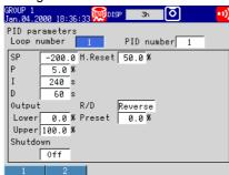
During ON/OFF control (when [Control] > [#5 Output processing] > [Control output] is set to [On/Off-control])
