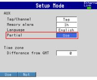
Detailed setting of the partial expanded display
